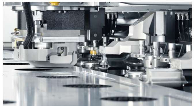
Retractable clamping claws ensure maximum utilization of each sheet.
